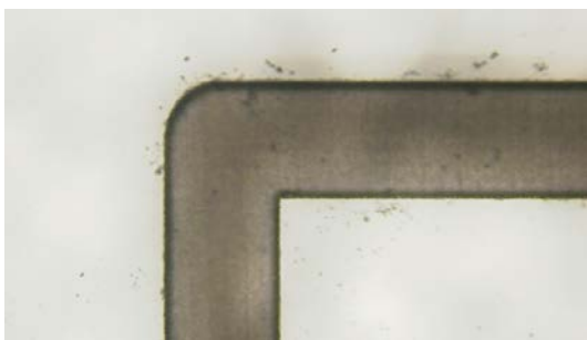
Figure 10: Optical view on detail of structured Borofloat® 33 before cleaning
